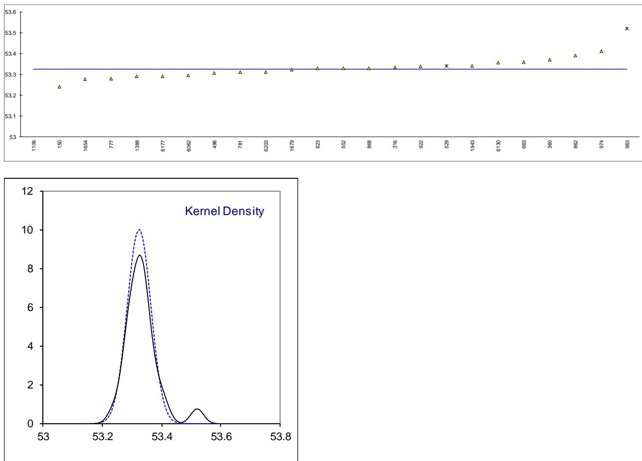
Determination of Caloric Value Superior or Gross Caloric Value (Real Gas, 101.325 kPa, combustion temperature 15°C, metering temperature 15°C) on sample #19060; results in MJ/m<sup>3</sup>
