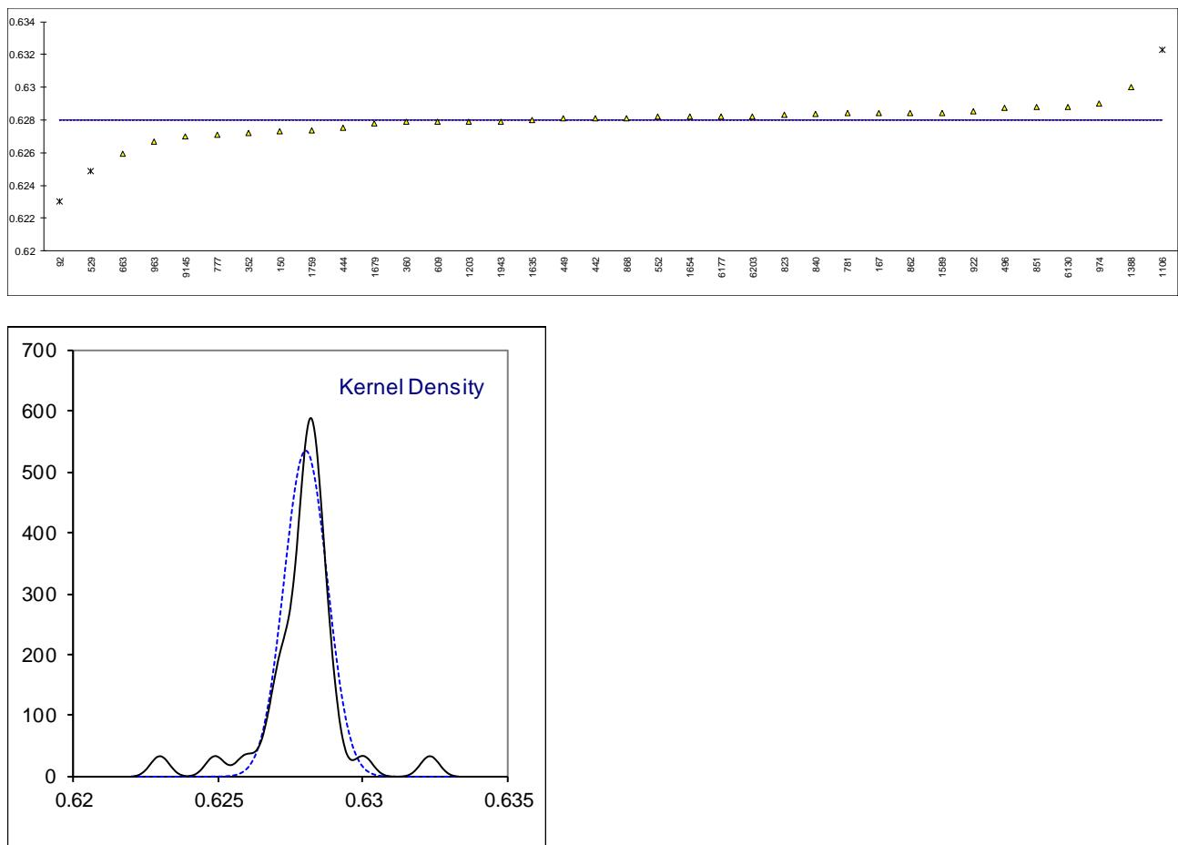
Determination of Wobbe Index (Real Gas, 101.325 kPa, combustion temperature 15°C, metering temperature 15°C) on sample #19060; results in MJ/m<sup>3</sup>
