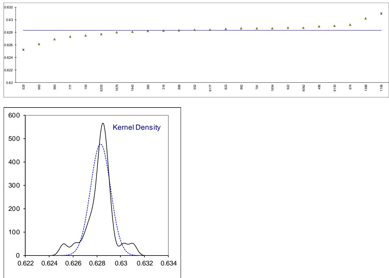
Determination of Wobbe Index (Real Gas, 101.325 kPa, combustion temperature 25°C, metering temperature 0°C) on sample #19060; results in MJ/m<sup>3</sup>
