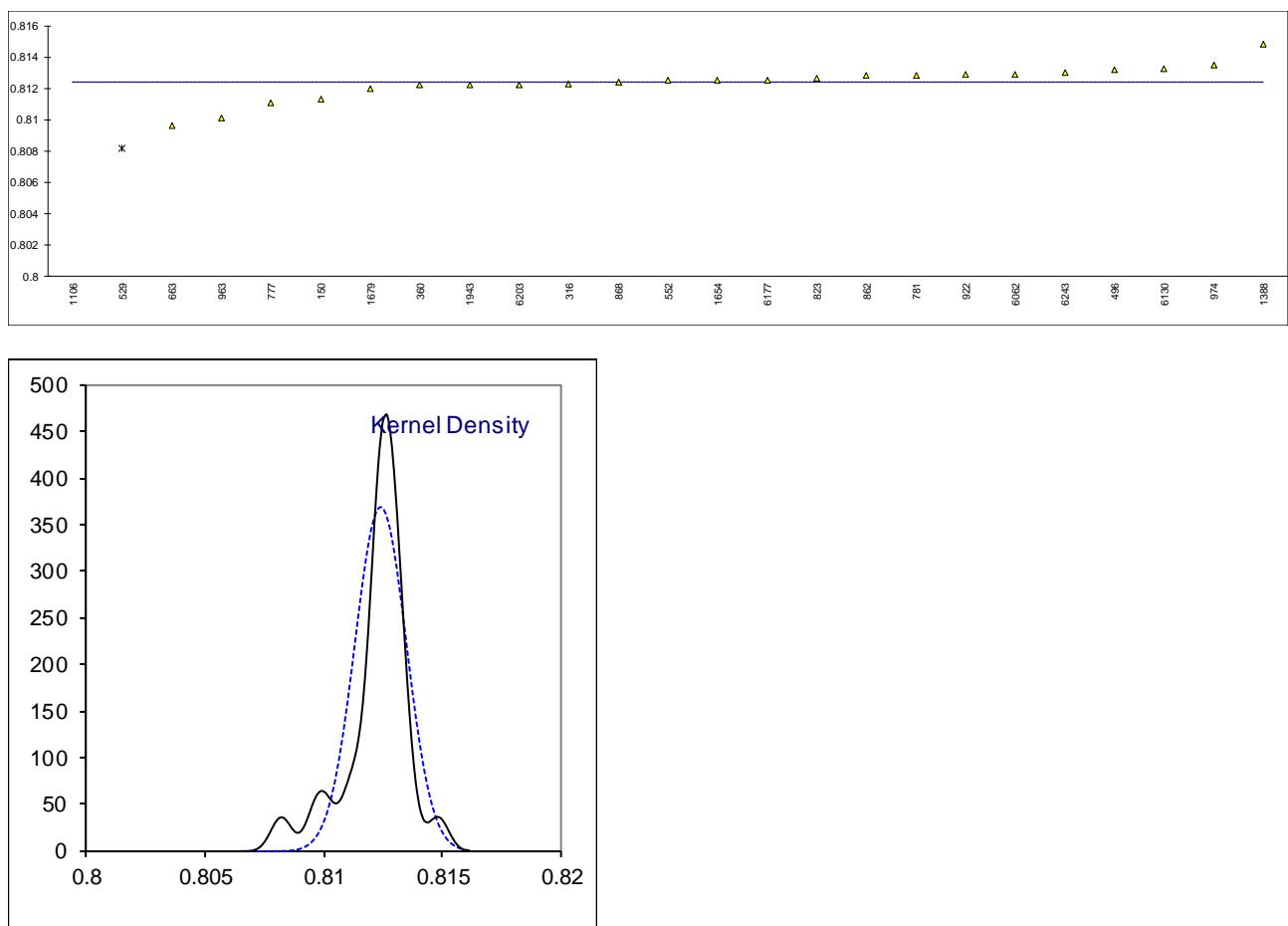
Determination of Relative Density (Real Gas, 101.325 kPa, combustion temperature 25°C, metering temperature 0°C) on sample #19060; results have no unit
