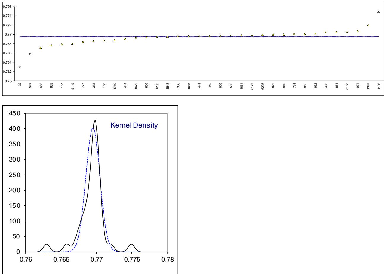
Determination of Relative Density (Real Gas, 101.325 kPa, combustion temperature 15°C, metering temperature 15°C) on sample #19060; results have no unit
