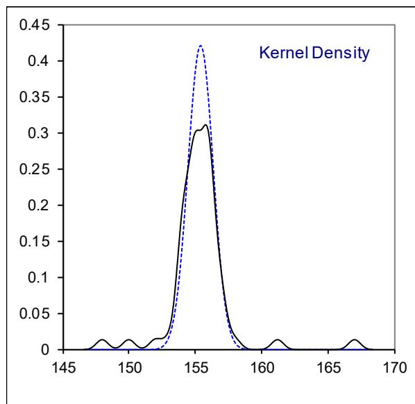
Determination of Viscosity Stabinger at 40°C on sample #19095; results in mm<sup>2</sup>/s
