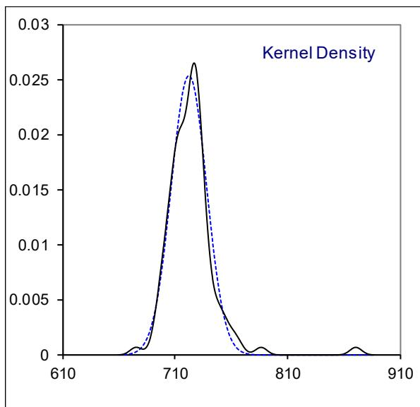
Determination of Kinematic Viscosity at 100°C on sample #19105; results in mm<sup>2</sup>/s
