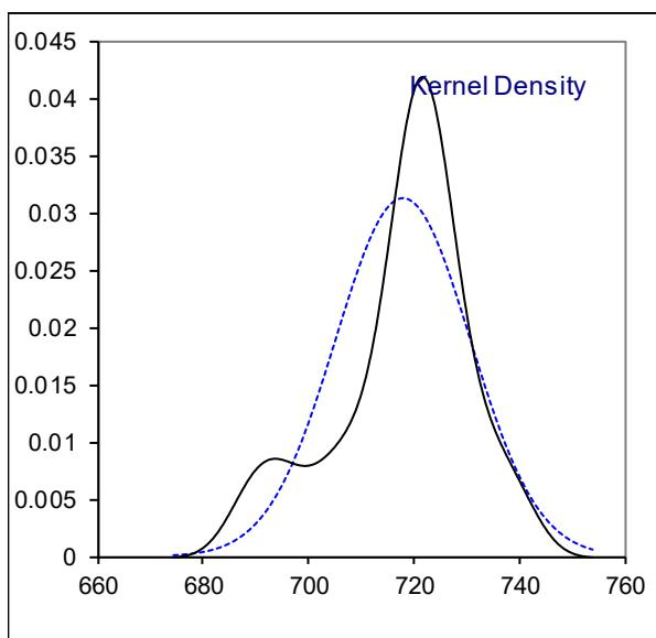
Determination of Viscosity Stabinger at 100°C on sample #19105; results in mm<sup>2</sup>/s
