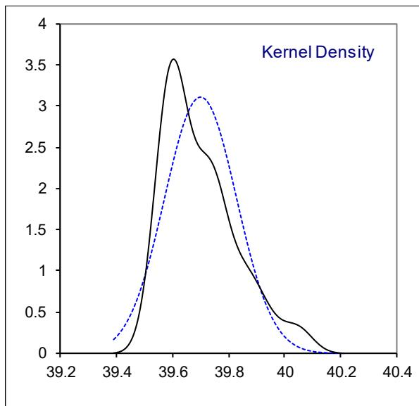
Determination of Kinematic Viscosity at 50°C on sample #19105; results in mm<sup>2</sup>/s
