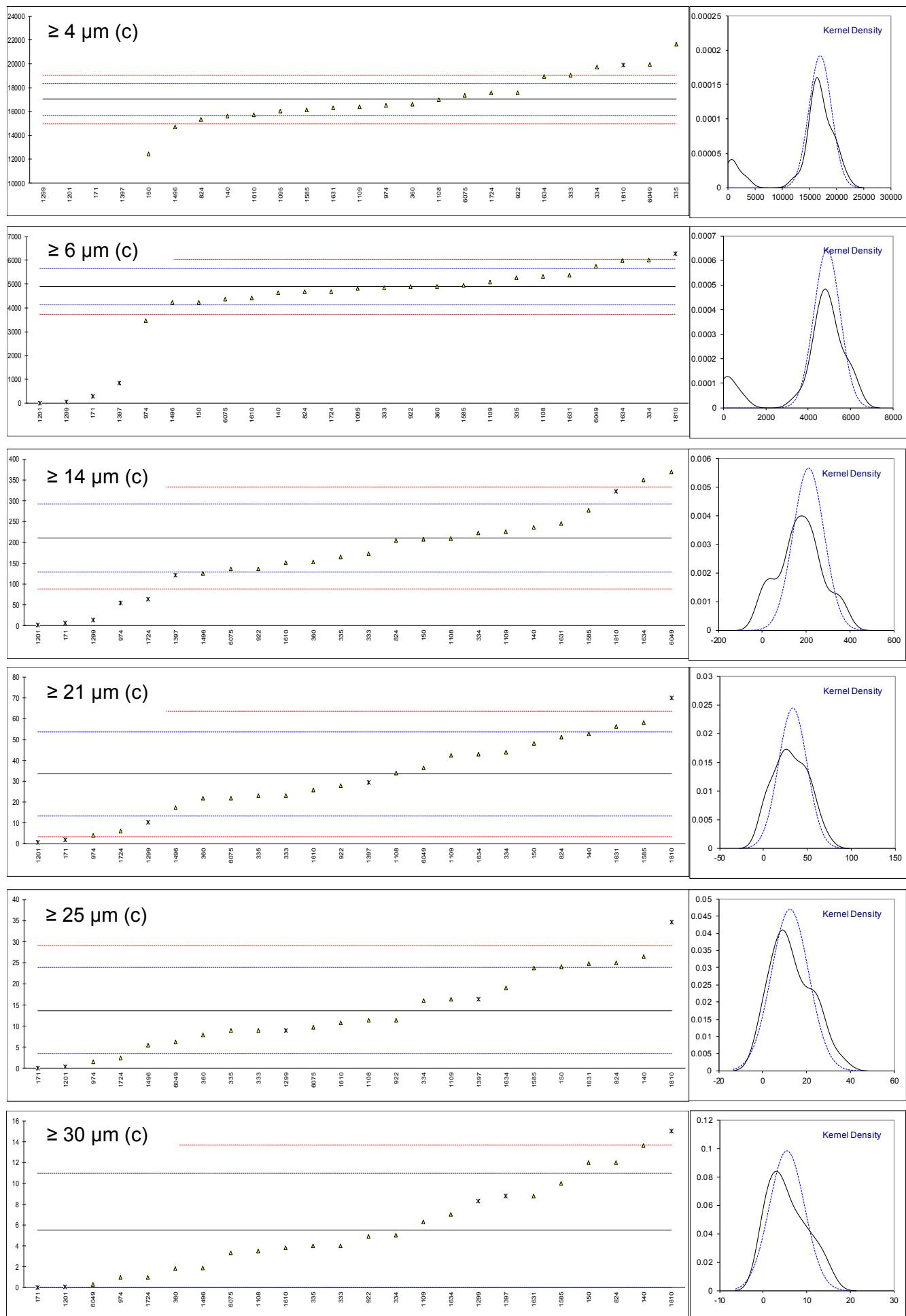
Determination of Particle Size Distribution by IP565 on sample #18031 acc. to ISO4406 scale, results in scale number
