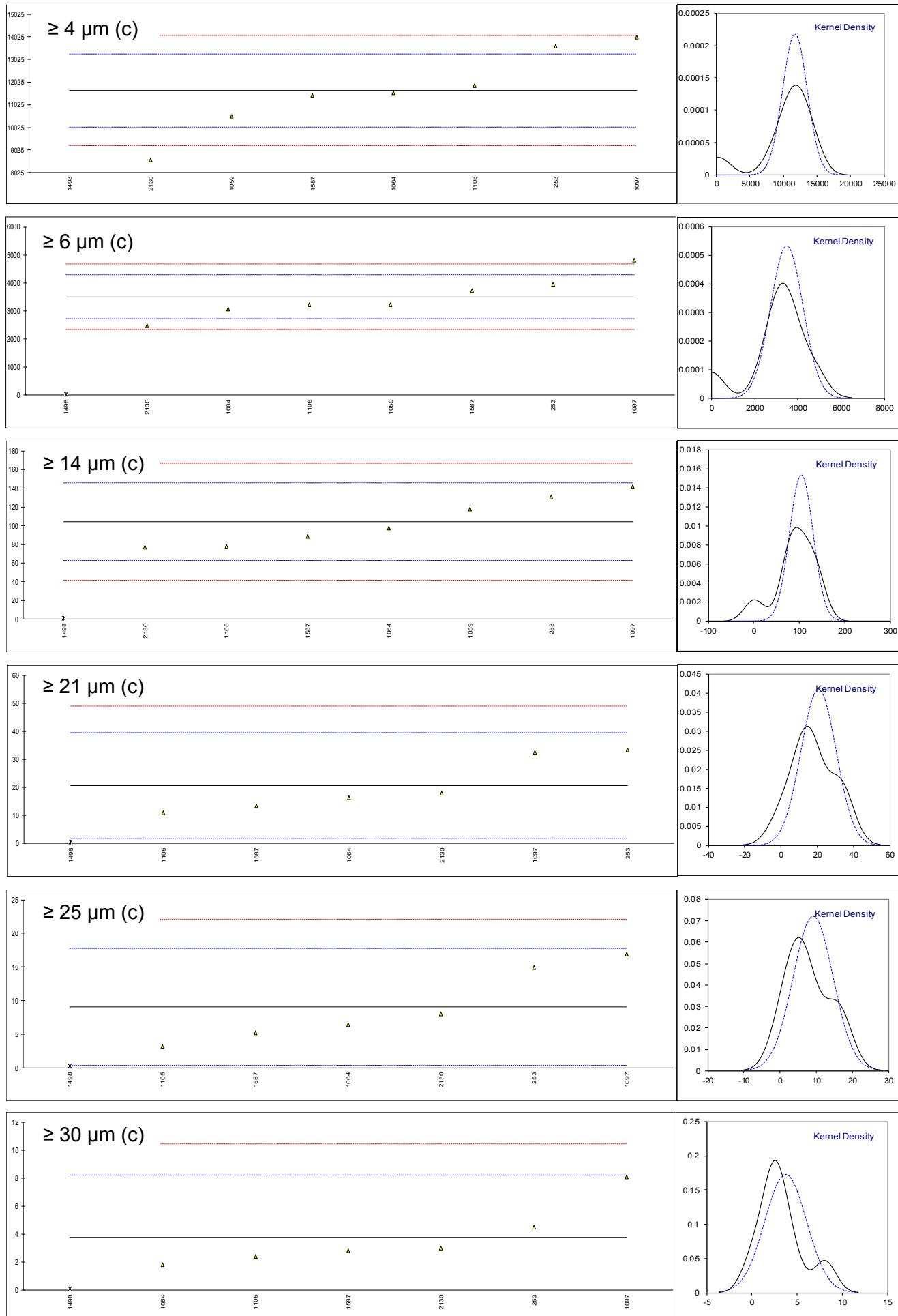
Determination of Particle Size Distribution by IP564 on sample #18031 acc. to ISO4406 scale, results in scale number
