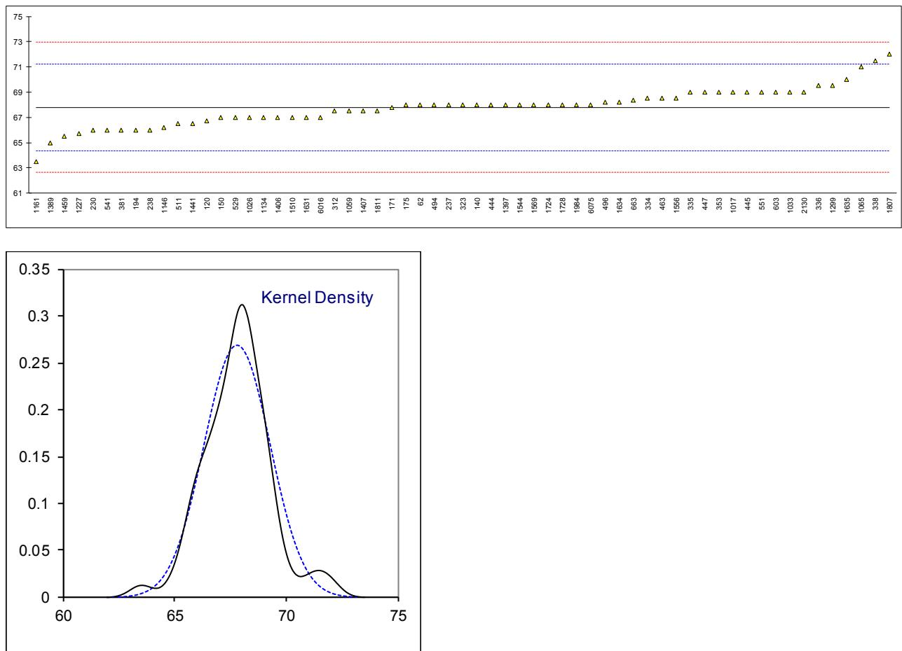
Determination of Kinematic Viscosity at 40°C on sample #18090; result in mm<sup>2</sup>/s
