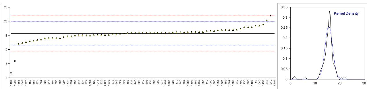
Determination of Bromine Number on distillate <360°C AET on sample #18267; results in g Br<sub>2</sub>/100g
