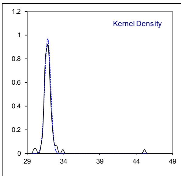
Determination of Viscosity Stabinger at 50°C on sample #18265; results in mm<sup>2</sup>/s
