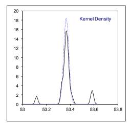
Determination of Caloric Value Superior (101.325 kPa, comb. temp. 15°C, metering temp 15°C) on sample #17040; results in M.I/m³ (real gas)
