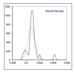
Determination of Wobbe Index (101.325 kPa , combustion temp. 25°C, metering temp. 0°C) on sample #17040; results in MJ/m³ (real gas)
