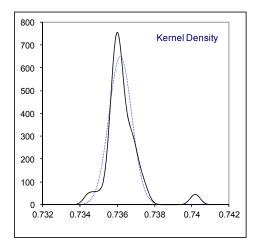
Determination of Relative Density (101.325 kPa, comb. temp. 15°C, metering temp. 15°C) on sample #17040; results have no unit (real gas)
