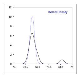
Determination of Caloric Value Superior (101.325 kPa, comb. temp. 25°C, metering temp 0°C) on sample #17040; results in MJ/m³ (real gas)
