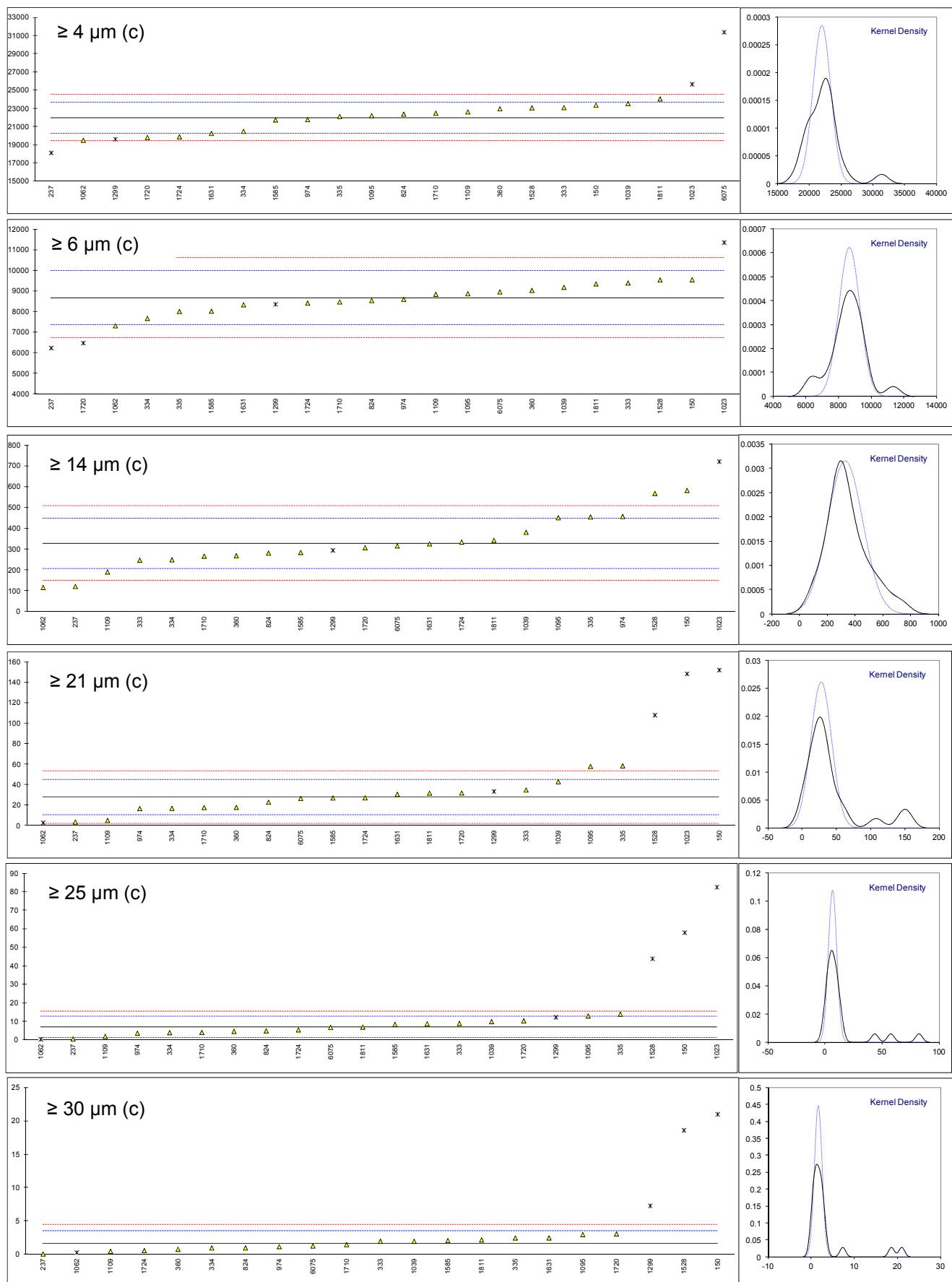
Determination of Particle Size Distribution by IP565 on sample #17031 acc. to ISO4406 scale, results in scale number
