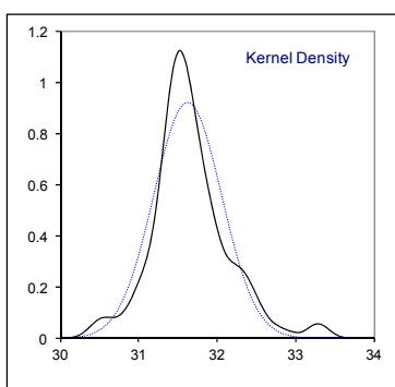
Determination of Viscosity Stabinger at 50°C on sample #17105; results in mm<sup>2</sup>/s
