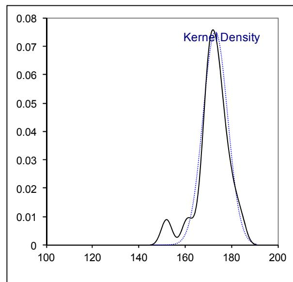
Determination of Iodine Value conform EN spec. on sample #16190; results in g I<sub>2</sub>/100g
