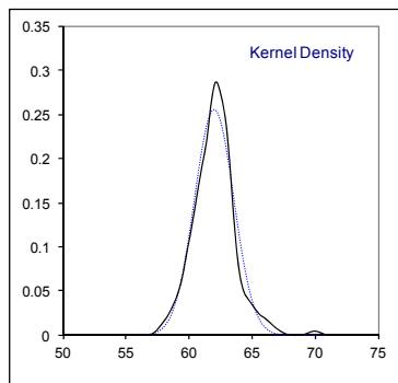
Determination of Kinematic Viscosity at 40°C, on sample #16180; results in mm<sup>2</sup>/s
