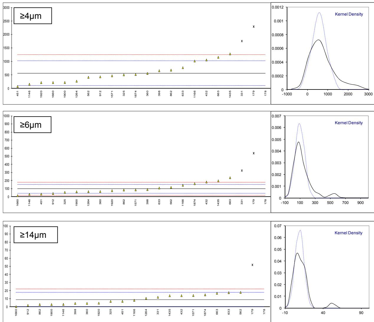
Determination of Level of Contamination acc. to ISO4406 scale on sample #16241; results in scale number
