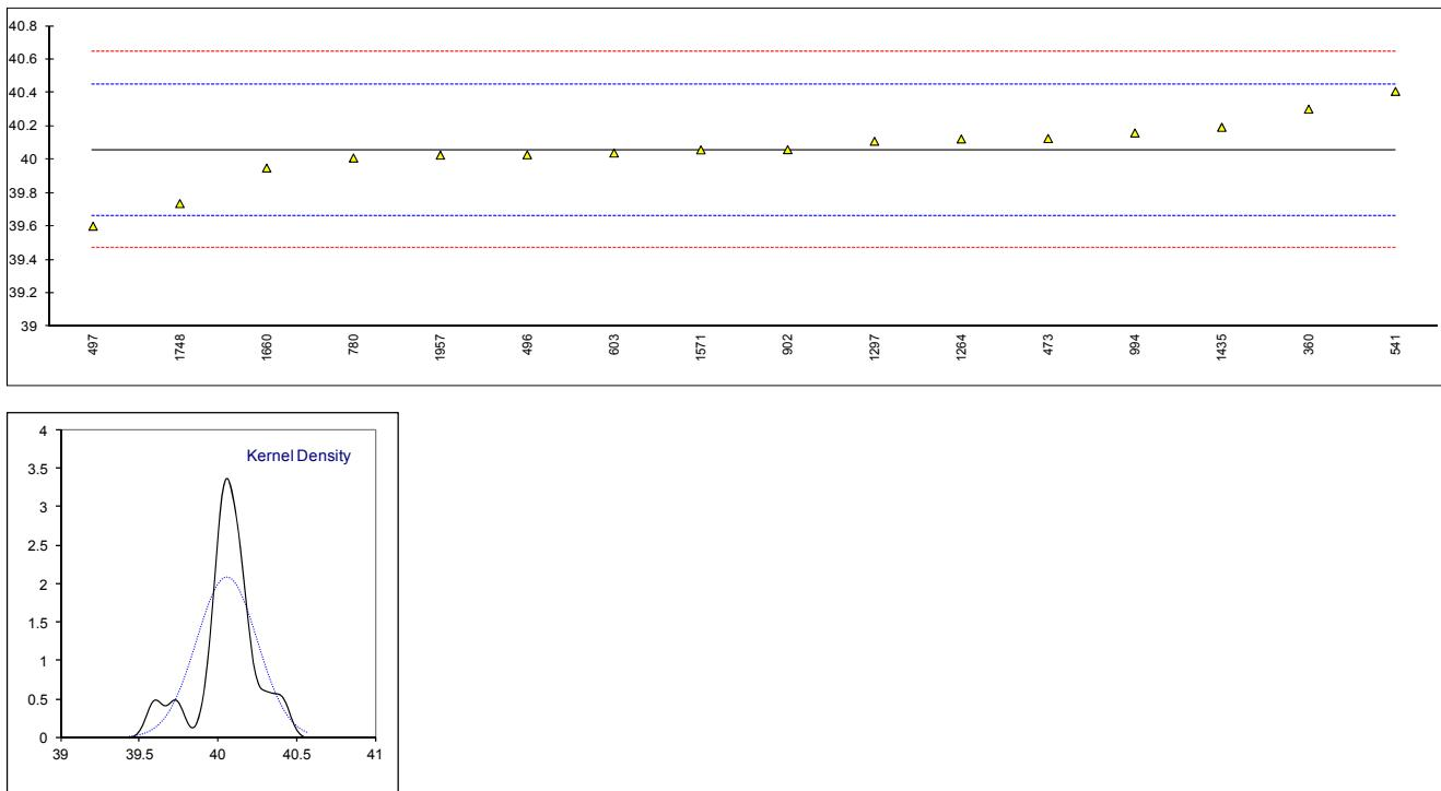
Determination of Viscosity Stabinger at 100°C on sample #16241; results in mm<sup>2</sup>/s.
