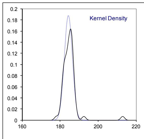
Determination of Kinematic Viscosity at 50°C on sample #16270; results in mm<sup>2</sup>/s
