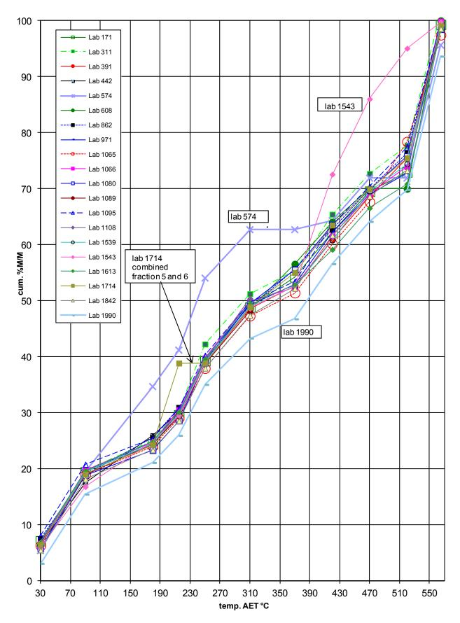
APPENDIX 3 True boiling point curve D2892, Sulphur in %M/M vs temp AET in °C
