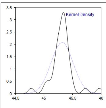
Determination of Kinematic Viscosity at 100°C on sample #15219; results in mm/s<sup>2</sup>
