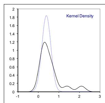
Determination of Particle Size Distribution on sample #15018 acc. to IP565, results in ml<sup>-1</sup>
