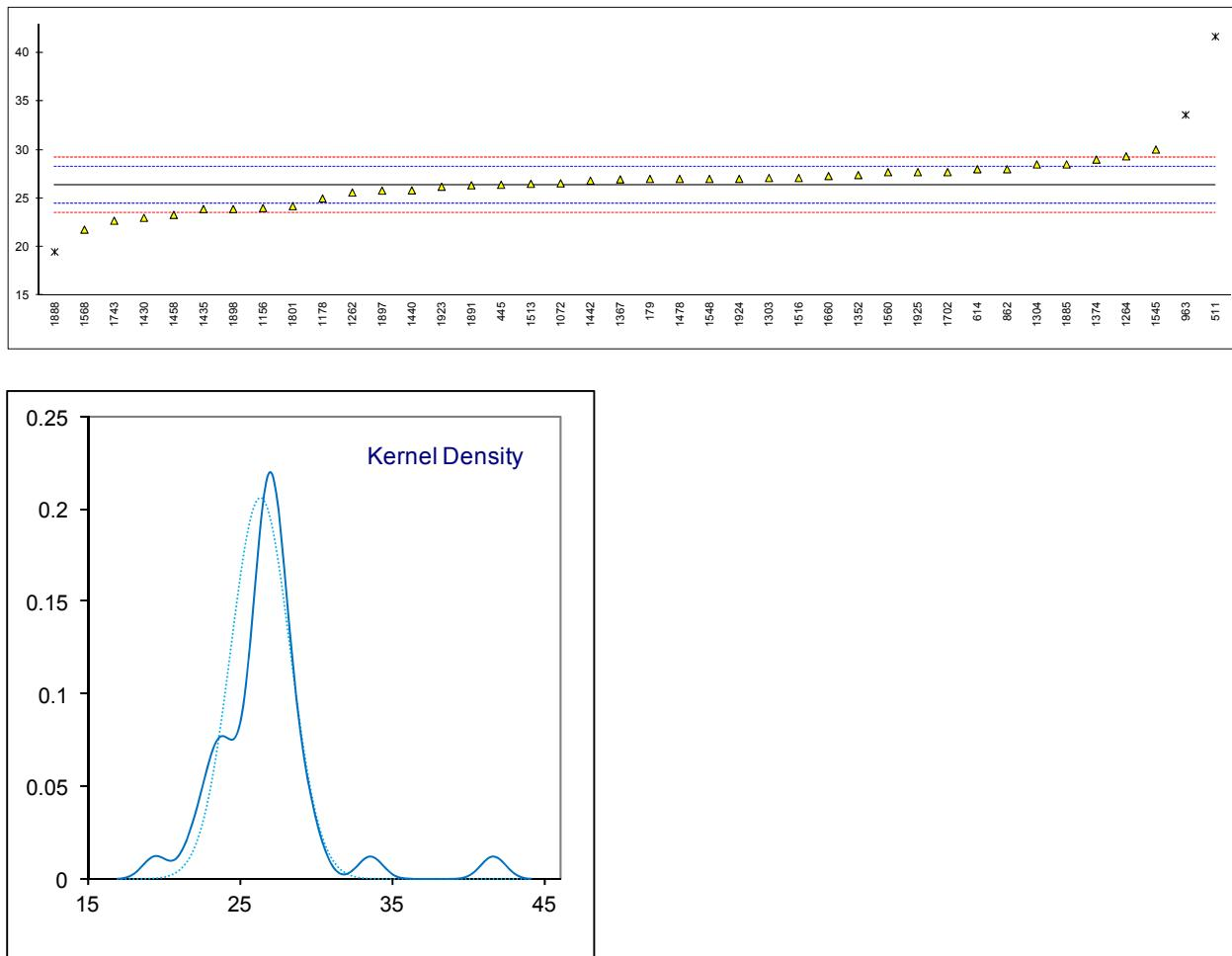
Determination of Kinematic Viscosity @ 40°C on sample #14223; results in mm<sup>2</sup>/s
