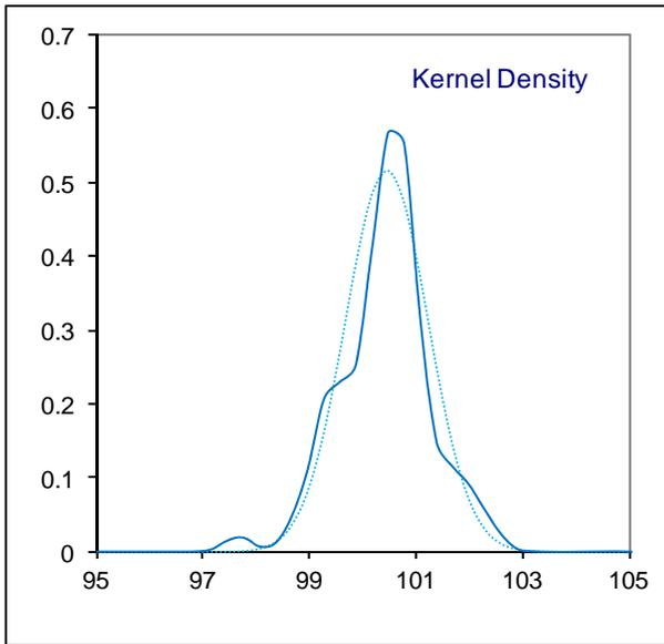
Determination of DVPE (acc. to EN13016-1) on sample #14196; results in kPa
