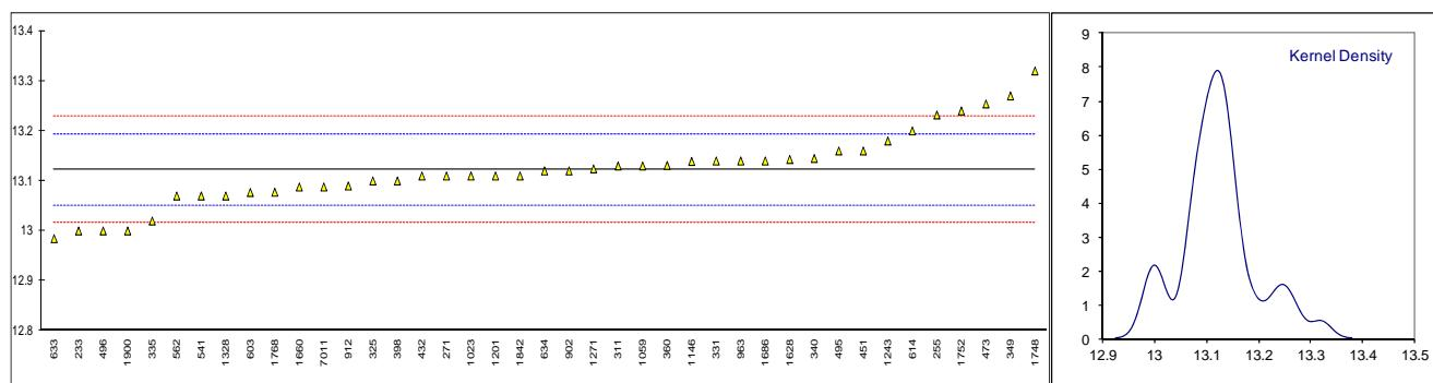
Determination of Kinematic Viscosity @ 100°C on sample #13204; results in mm/s<sup>2</sup>
