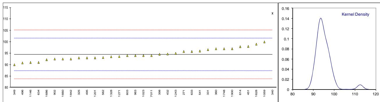
Determination of Kinematic Viscosity @ 40°C on sample #13204; results in mm/s<sup>2</sup>.
