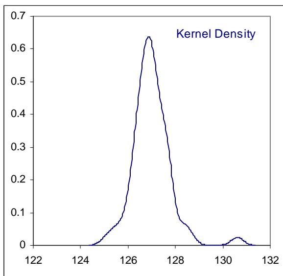
Determination of Kinematic Viscosity @ 100°C on sample #12063; results in mm<sup>2</sup>/s
