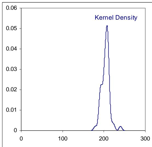
Determination of Kinematic Viscosity @ 40°C on sample #12063; results in mm<sup>2</sup>/s
