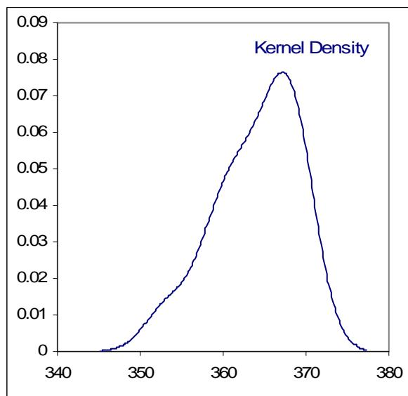
Determination of Viscosity Stabinger @ 100°C on sample #12001; results in mm<sup>2</sup>/s
