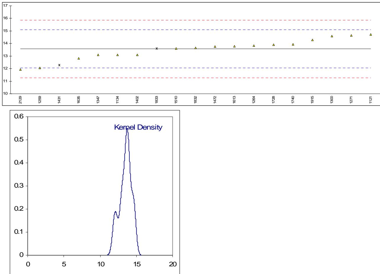
Determination of Density @ 15 °C on sample #12001; results in kg/m<sup>3</sup>
