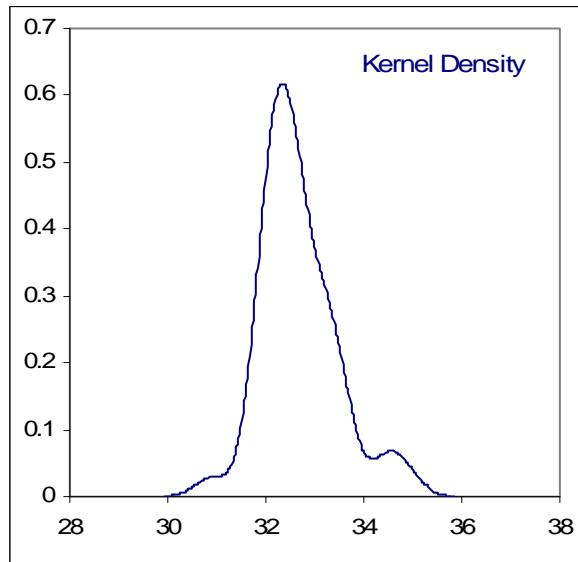
Determination of Viscosity Stabinger @ 50°C on sample #12001; results in mm<sup>2</sup>/s
