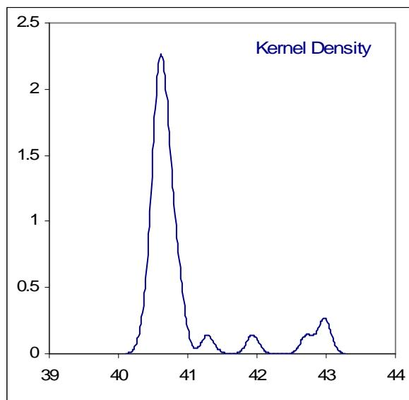
Determination of Kinematic Viscosity @ 50°C on sample #12001; results in mm<sup>2</sup>/s
