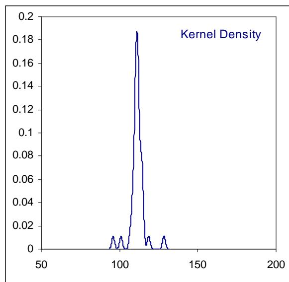
Determination of Kinematic Viscosity @ 40°C on sample #11036; results in mm<sup>2</sup>/s
