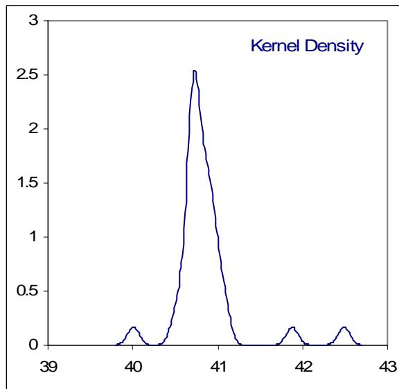
Determination of Kinematic Viscosity @ 50°C on sample #11001; results in mm<sup>2</sup>/s
