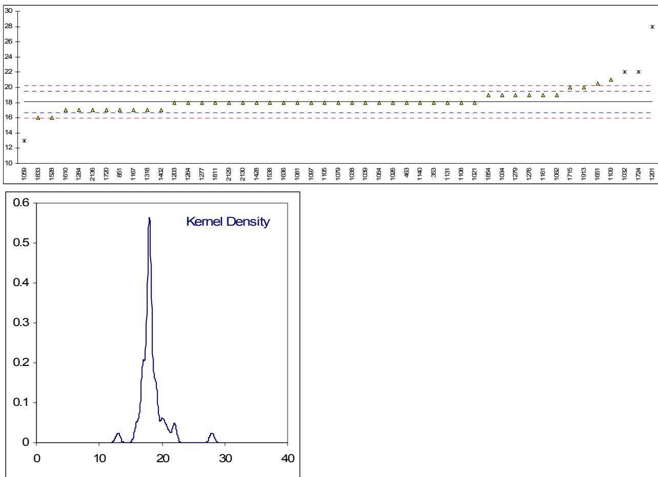
Determination of Density @ 15°C on sample #1017; results in kg/m<sup>3</sup>
