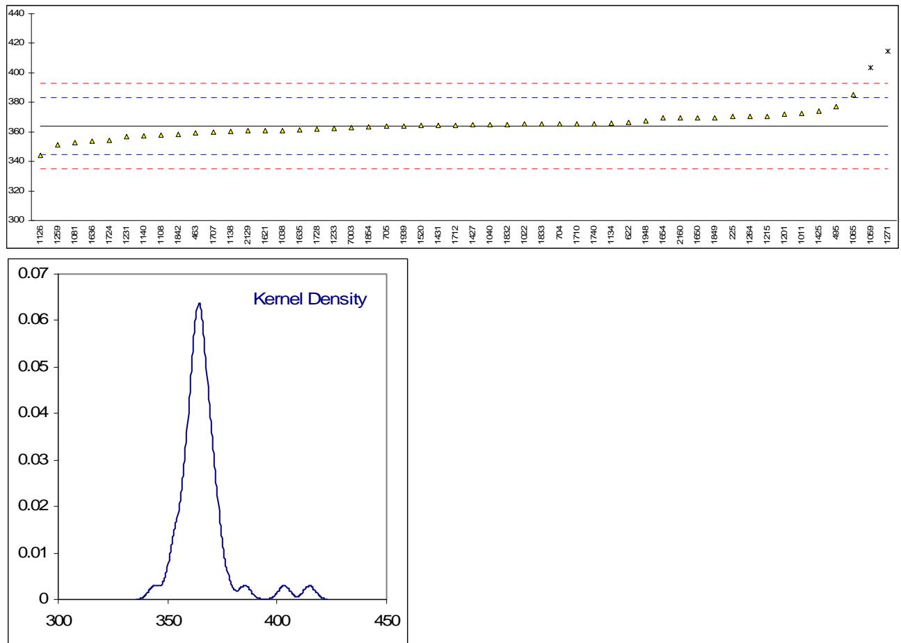
Determination of Kinematic Viscosity @ 100°C on sample #1003; results in mm<sup>2</sup>/s
