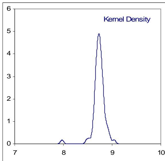
**APPENDIX 2****z-scores distillation ASTM D86 (automated mode)**
